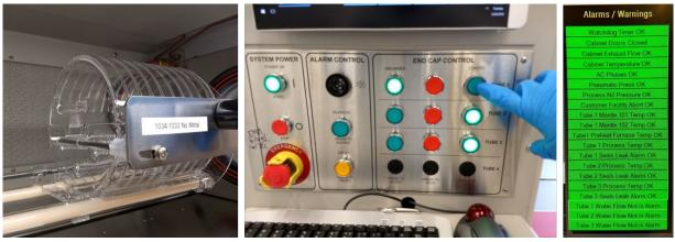
4.10 Make sure the recipe is completed and Tube is left in Initial Conditions by checking the status of Tube Panel: "Setup – Initial Conditions".
