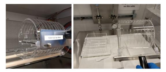
3.5 To load the wafers, place the wafers edgewise into the holding slots of the quartz boat so that they face perpendicular to the direction of the loading arm motion. Do not use metal tweezers but PTFE (Teflon) tweezers when transferring wafers.
