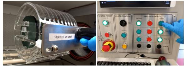
3.8 Wait until the door are closed and "Seals Leak Alarm" on Alarm Panel is satisfied and solid GREEN
